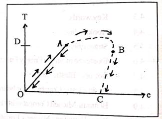
is removed, the line BC is retraced, not the curve BAO, so that there is a permanent extension or plastic strain OCafter the removal of T. In this case rod does not fully recover its original length completely. The rod exhibits plasticity.
