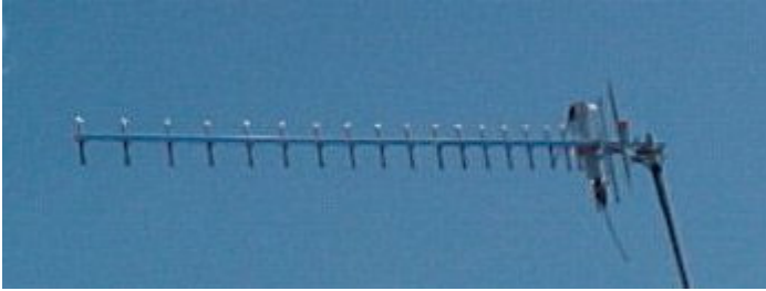
Figure 7. - a vertically polarised UHF Yagi antenna
