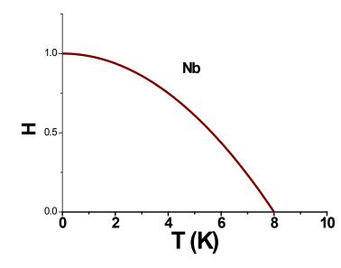
Critical temperature for Niobium(Nb) is shown in figure. We note that the curves are nearly parabolic can reasonably represented by
