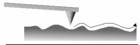
Figure 7: In contact mode AFM the probe directly follows the topography of the surface as it is scanned. The force of the probe is kept constant while an image is measured.
