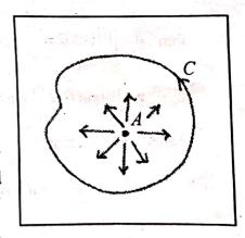
Thus if  $2\pi m$  is the total volume of flow across any small circle surrounding the source, then  $m_{is}$  called strength of the source. Sink is a source of strength (-m).
