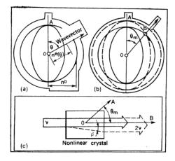
$n^{e}(\theta)$ . The extraordinary wave is polarized in the plane passing through the wave vector and the optic axis (exactly this plane is shown in Figure a), whereas the ordinary wave is polarized normally to this plane. The section through the surfaces of refractive index, shown in figure a, corresponds to a certain frequency of the incident light. Suppose now
